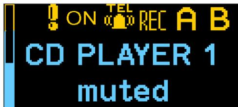
On the left of the OLED is a meter bar that gives you an indication of the input level,
